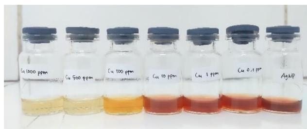
**Figure 8.** Colorimetric test of various concentrations of  $\text{Cu}^{2+}$
