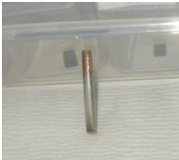
Figure 1. CoNi synthesis results using a copper wire substrate with the addition of boric acid.
