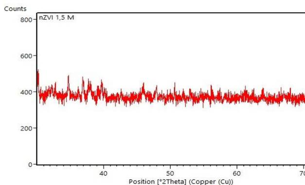
**Figure 6.** XRD diffractogram of ZVI sample
