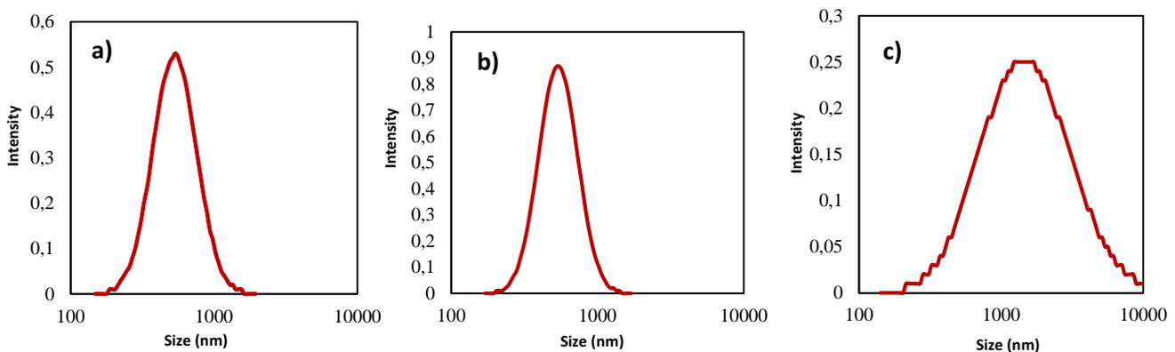
**Figure 4.** Graph of PSA particle size distribution based on intensity to the effect of feeding time a) 0 minutes; b) 30 minutes; c) 60 minutes
