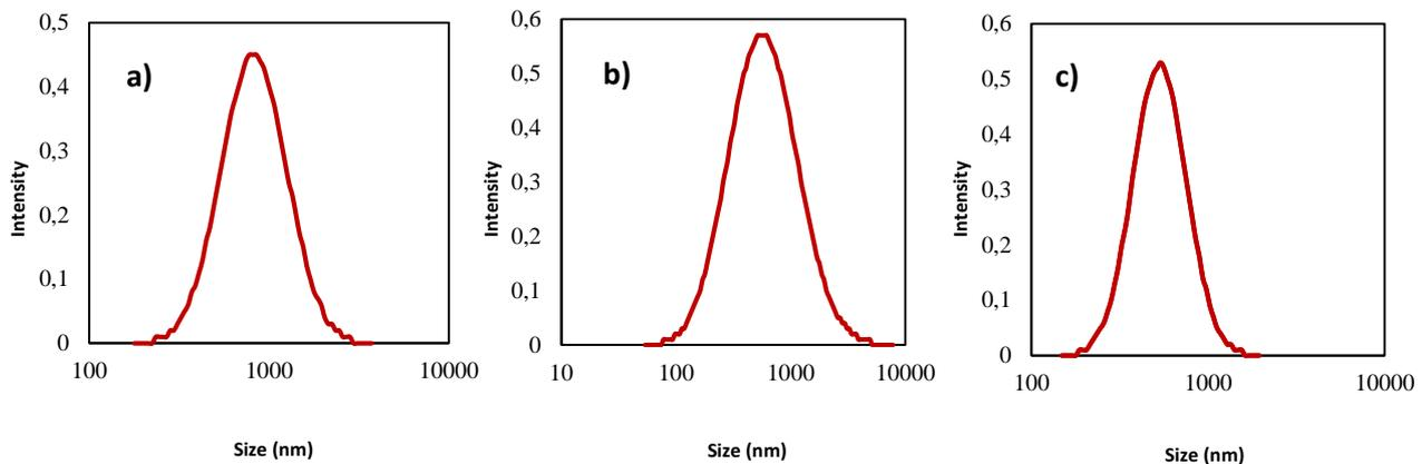
**Figure 3.** Graph of PSA particle size distribution based on intensity to effect of reaction temperature a) 0 °C; b) 10 °C; c) 25 °C
